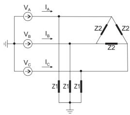
Dados:  $V_A = 120 \angle 0^{\circ} V$ ;  $V_B = 120 \angle -120^{\circ} V$ ;  $V_c = 120 \angle 1200^{\circ} V; Z_1 = 10 \angle 30^{\circ} \Omega$  $e Z_2 = 15 \angle 30^{\circ} \Omega$
