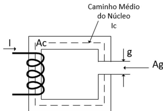
(A)  $R_c = \frac{4,8 \times 10^{-3}}{4 \times \pi \times 10^{-7}} \frac{A \times e}{Wb}$ ,  $R_g = \frac{0,6}{4 \times \pi \times 10^{-7}} \frac{A \times e}{Wb}$ ,  $\varphi = 9 \times 10^{-4} \text{ Wb}$ .
