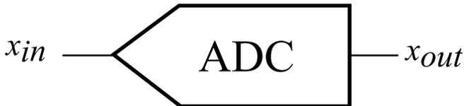
The output of a microphone, the voltage at a photodiode or the signal of an accelerometer are examples of analog values that need to be converted so that a microprocessor can work with them.
